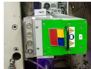
UV Ray's MaxLED curing system on Skanem India's Gidue E-Combat press
