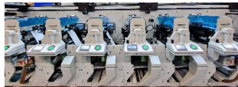
Eurolabel's Lombardi press with UV Ray's MaxLED curing systems
